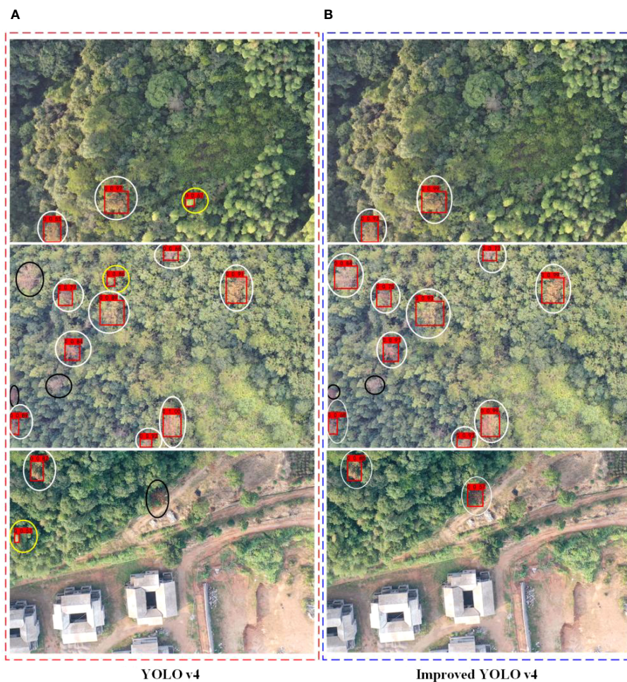
FIGURE 12 Remote sensing image recognition results under strong light environment. * white circles indicate correct detections, black circles indicate missed detections, yellow circles indicate misdetections. (A) YOLO v4 detection results (B) Improved YOLO v4 detection results.
