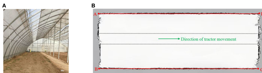
FIGURE 13 Greenhouse environments and maps created by the Gmapping algorithm. (A) Greenhouse environment. (B) Map created by Gmapping algorithm.
