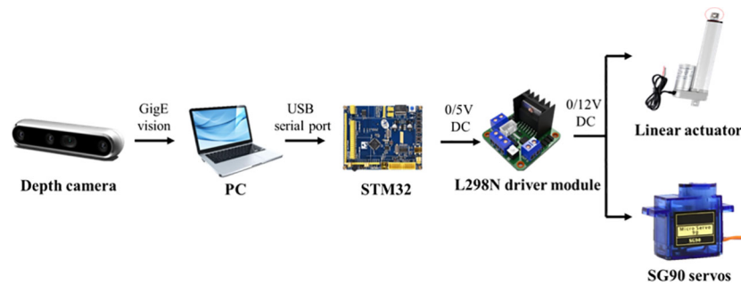
FIGURE 6 Orientation control system composition.
