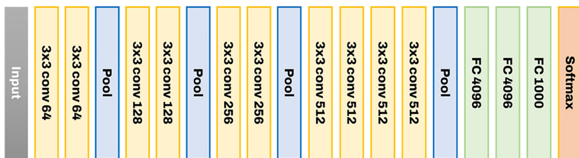
FIGURE 3 The structure of VGGnet-19 used to develop the image classification model.
