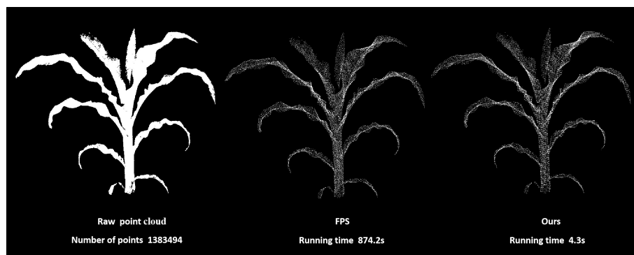
FIGURE 2 A comparison plot of plant point cloud down-sampling methods.
