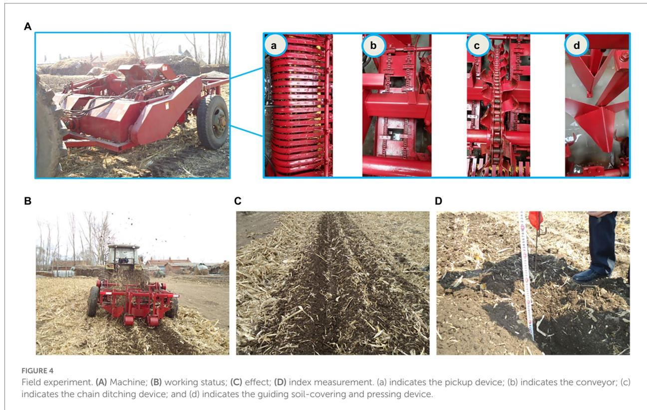
**FIGURE 4** Field experiment. (A) Machine; (B) working status; (C) effect; (D) index measurement. (a) indicates the pickup device; (b) indicates the conveyor; (c) indicates the chain ditching device; and (d) indicates the guiding soil-covering and pressing device.
