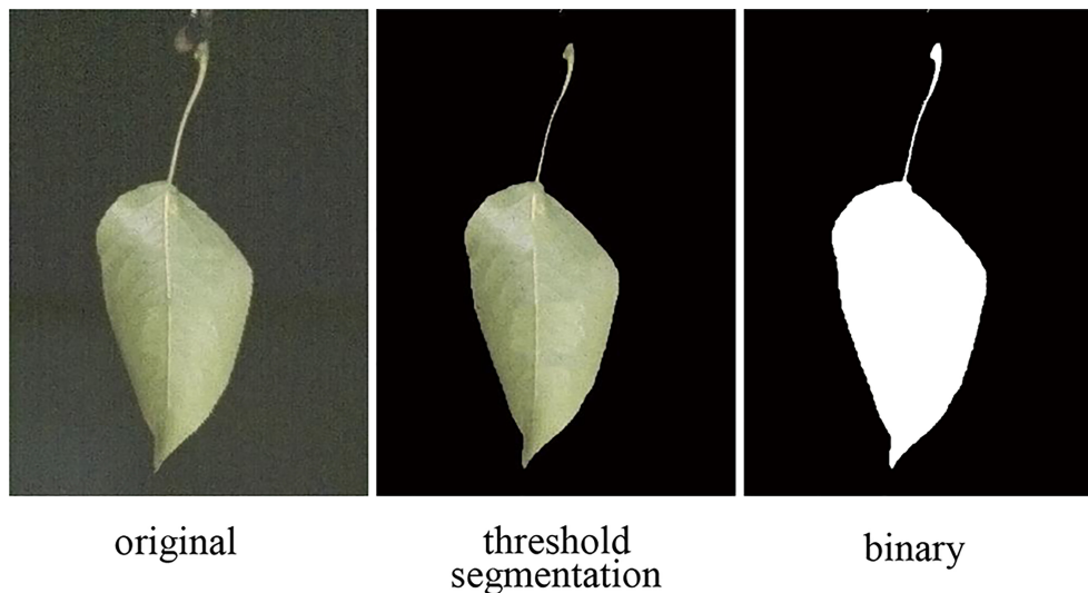
FIGURE 4 Image processing to obtain the wind deflection area of the leaf.
