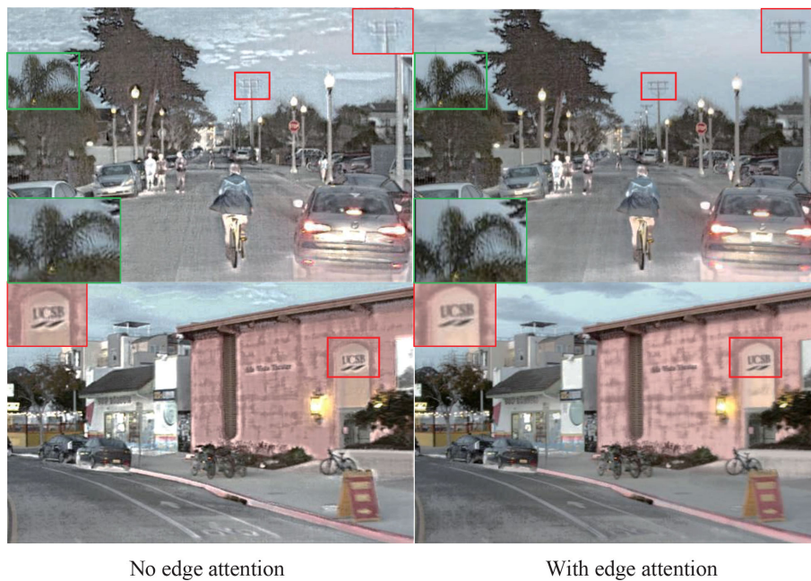
FIGURE 10 The results of ablation study about the influence of edge attention module in two image pairs from the Roadscene dataset.
