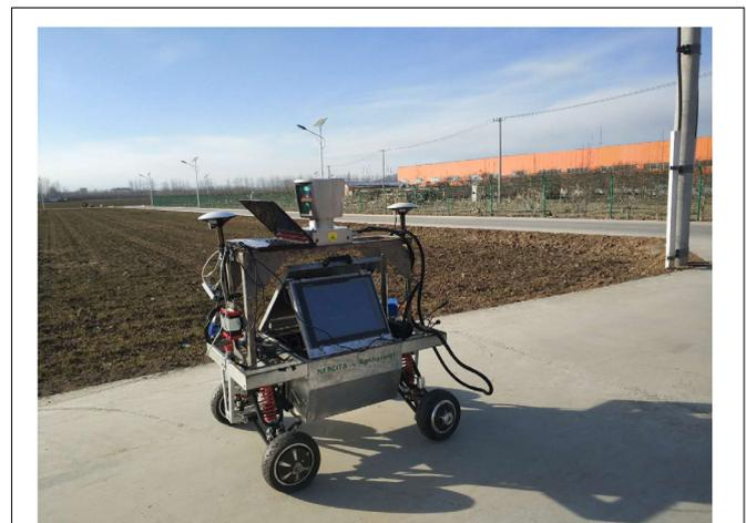
**FIGURE 1** | Velodyne HDL64E-S3 on the robot.
