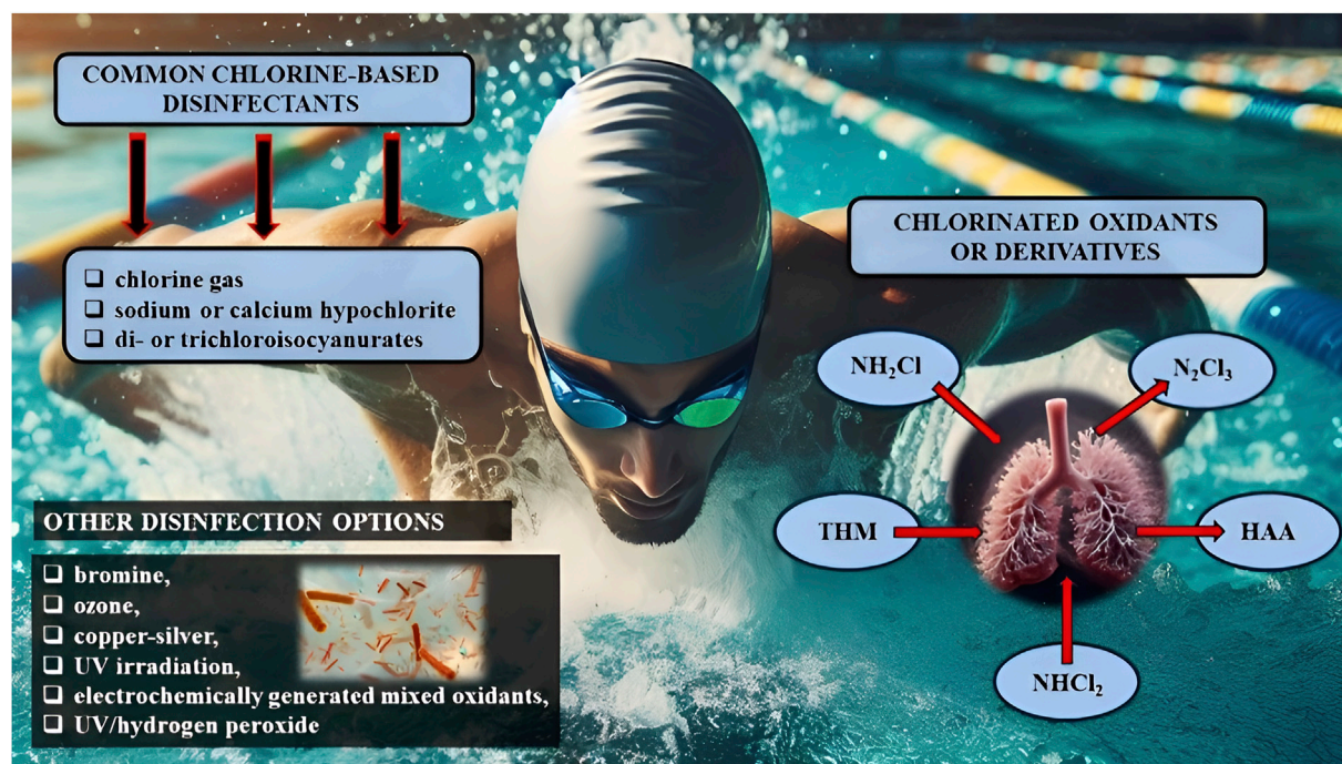
FIGURE 1 Chlorine-based disinfectants commonly used in indoor pools and swimmers' exposure to chlorinated oxidants/derivatives that can be inhaled, ingested or absorbed through the skin. Note: \text{NH}_2\text{Cl} , monochloramines; \text{NHCl}_2 , dichloramines; \text{N}_2\text{Cl}_3 , trichloramines; THM, trihalogenomethanes; HAA, haloacetic acid; UV, ultraviolet.
