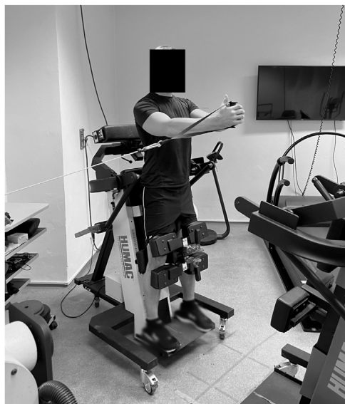
FIGURE 1 Maximal voluntary contraction test of trunk rotational strength using isometric mode of Humac NORM dynamometer with Trunk Modular and Wheel Components (CSMi, Stoughton, MA).
