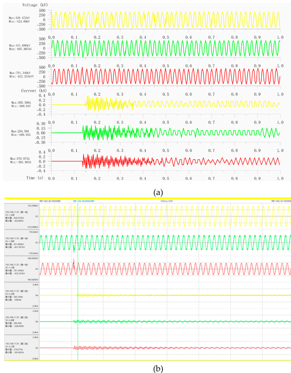
FIGURE 16 Bus voltage and branch current while switching off reactive power compensation. (A) Wireless synchronous acquisition system; (B) on site.
