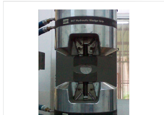
FIGURE 1 MTS machine loads the Brazilian disk.
