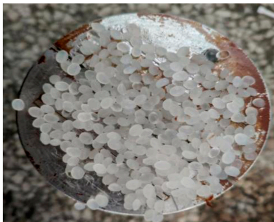
FIGURE 7 Accumulation of 10/40 mesh granular temporary plugging agent at the fracture opening.
