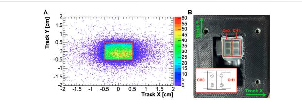
(A): Extrapolation of tracks to the upstream crystal face and localisation of the geometrical  $1 \times 1$  cm<sup>2</sup> fiducial volume (red). (B): Photo of Proto-0 assembly. The PbF<sub>2</sub> crystal and SiPM matrix are visible (the front wrapping was removed). The SiPM series wiring scheme is shown in the inset and the tracking coordinate system in overlay.
