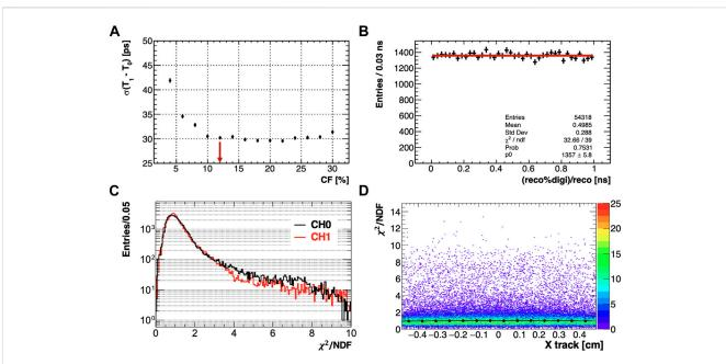
Timing reconstruction diagnostics. (A): Example of constant fraction optimisation by minimisation of the timing resolution. (B): Plot of reconstructed time modulo the digitiser sampling period of 200 ps, showing no significant bias from the timing algorithm. (C): Example of  $\chi^2$  distributions resulting from template fits applied to PbF<sub>2</sub> waveforms for CH0 (black) and CH1 (red). (D):  $\chi^2$  distribution as a function of the particle hit position on the crystal.
