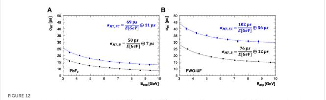
Mean-time resolution of a single calorimeter cell for PbF<sub>2</sub> (A) and PWO-UF (B) as a function of  $E_{dep}$  over the range 3–10 GeV. Front-configuration corrected runs ( $\sigma_{MT,EC}$ ) are shown in blue, while back-configuration runs ( $\sigma_{MT,E}$ ) are shown in black.
