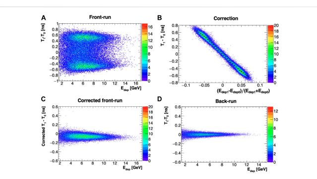
Overview of the procedure for the correction of position-dependent effects for evaluation of the timing performance. (A): Time difference between the two readout channels as a function of  $E_{dep}$ , for front configuration runs. The splitting of the distribution from position-dependent effects is evident. (B): Timing correction using charge asymmetry. Bottom: Distributions for runs in front (C) and back (D) configurations.
