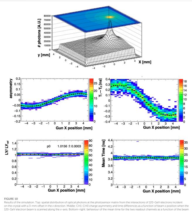
120-GeV electron beam is scanned along the x-axis. Bottom-right: behaviour of the mean time for the two readout channels as a function of the beam position. Bottom-left: behaviour of the mean charge response as a function of the beam position, using the normalized light yield LY/LY<sub>ref</sub>, where LY is the mean value of p. e./MeV for the two readout channels at a given beam position, and  $LY_{ref}$  is the mean LY obtained with the centred beam. A constant function fit (p0) is overlaid.
