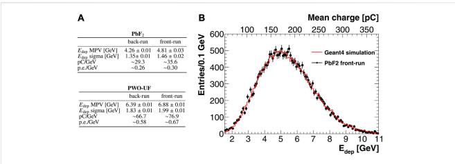
Determination of the energy scale. (B): example of data-MC overlay for energy deposit fit for PbF<sub>2</sub> front. (A): Summary of energy scale and relative parameters for the two crystals in both run configurations. The values of MPV( $E_{dep}$ ) and  $\sigma(E_{dep})$  were obtained via fits to a Gaussian-convoluted Landau distribution.
