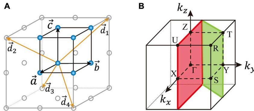
**FIGURE 1** (A) Unit cell (black frame and blue balls) and hopping vectors  $\vec{a}$ ,  $\vec{b}$ ,  $\vec{c}$ , and  $\vec{d}_i$  ( $i = 1, 2, 3, 4$ ) of the model. (B) Bulk BZ and its projections to the (010) surface (red) and (110) surface (green).
