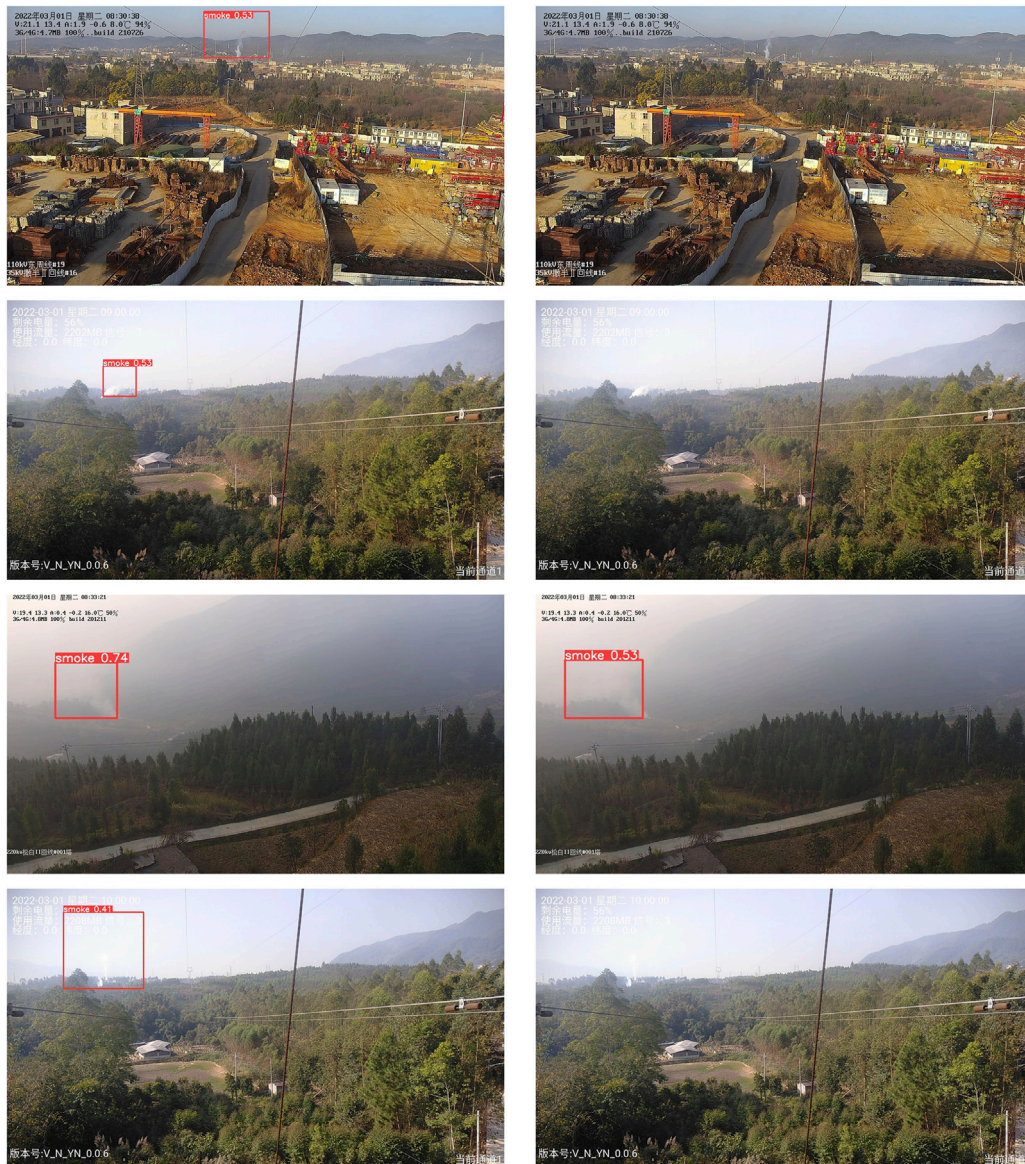
FIGURE 6 Detection result display. The left is the result of the proposed method, and the right is the result of baseline.
