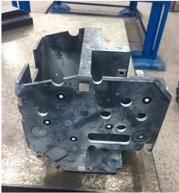
FIGURE 5 Schematic diagram of the precision machined workpiece and pasting mark points.
