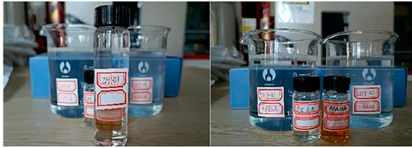
FIGURE 7 | Compatibility test of the foaming agent and scale inhibitor.
