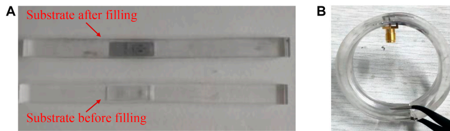
FIGURE 4 | Photographs of the fabricated wearable antenna. (A) Flat wristband before and after filling LM and (B) curved wristband filled with LM.
