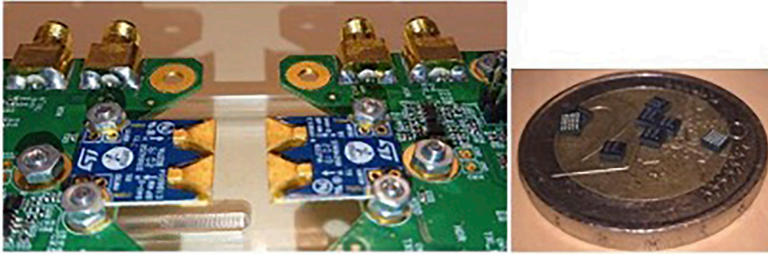
FIGURE 2 | ST Microelectronics ST60 contactless connectivity transceiver in BGA.
