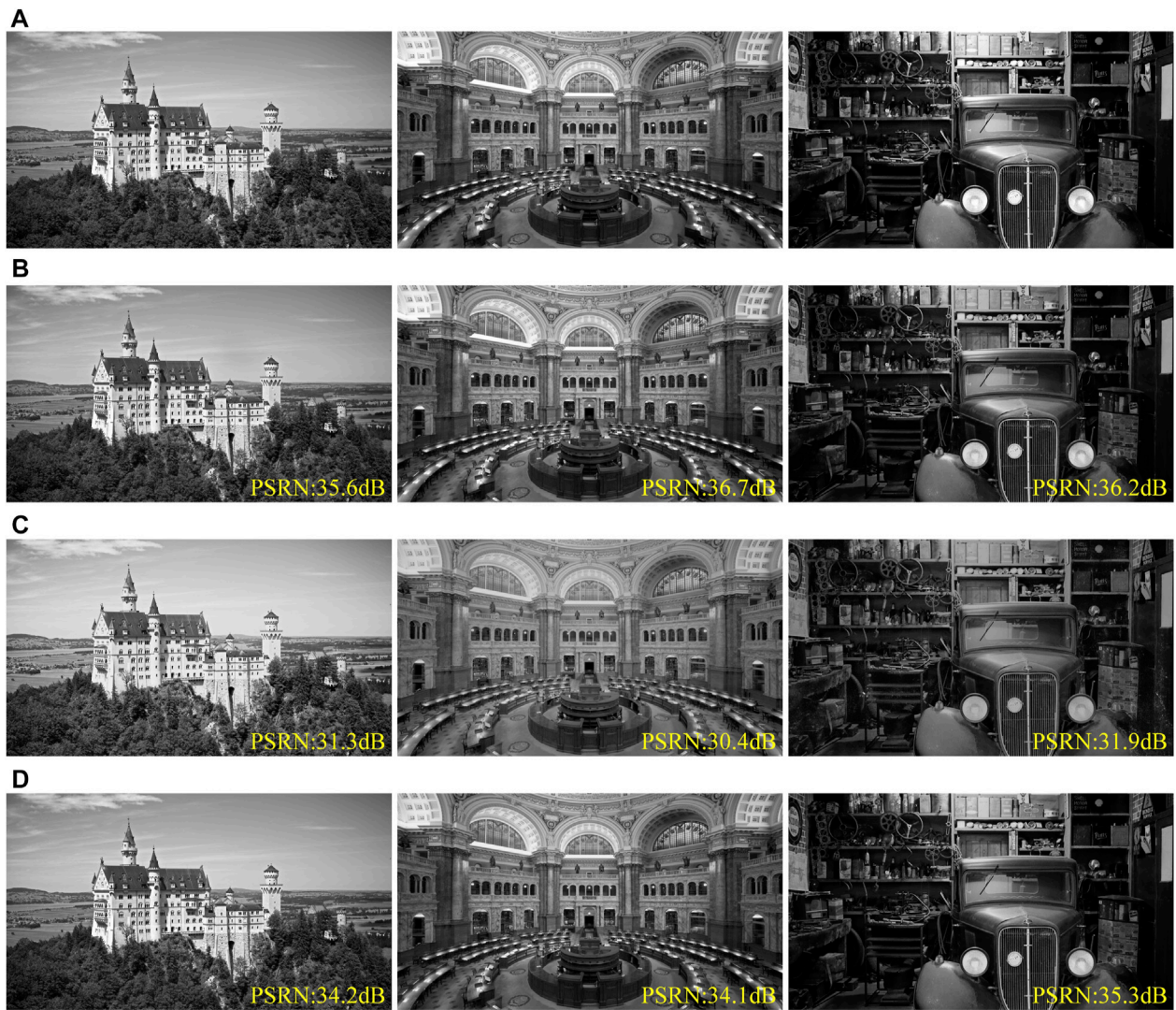
FIGURE 10 Numerical reconstructed images of phase-only holograms generated by different methods. (A) Target images, (B) WH, (C) DPH, and (D) the proposed method.
