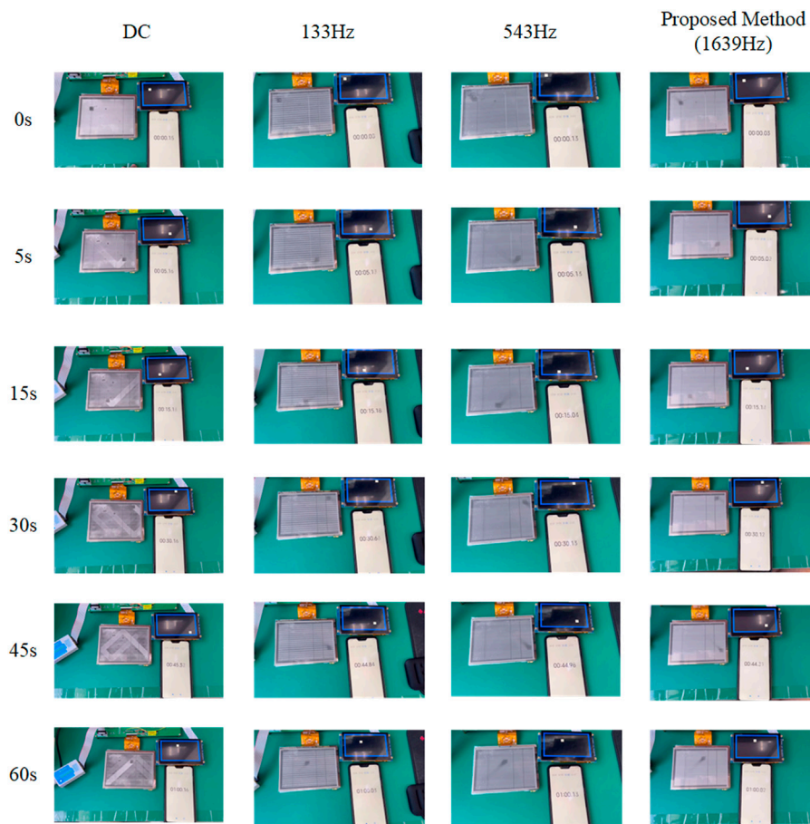
FIGURE 12 Asymmetric AC driving results at different frequencies.
