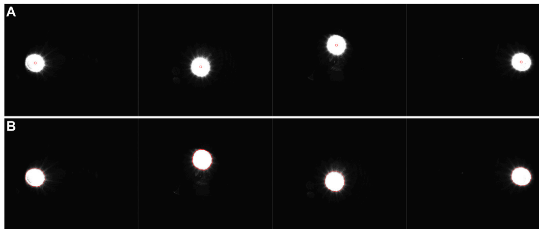
FIGURE 4 Adaptive initial curve coordinates and evolutionary results. (A) : Images of laser spot at different positions; (B) : Fitting results of laser spot images at different positions.
