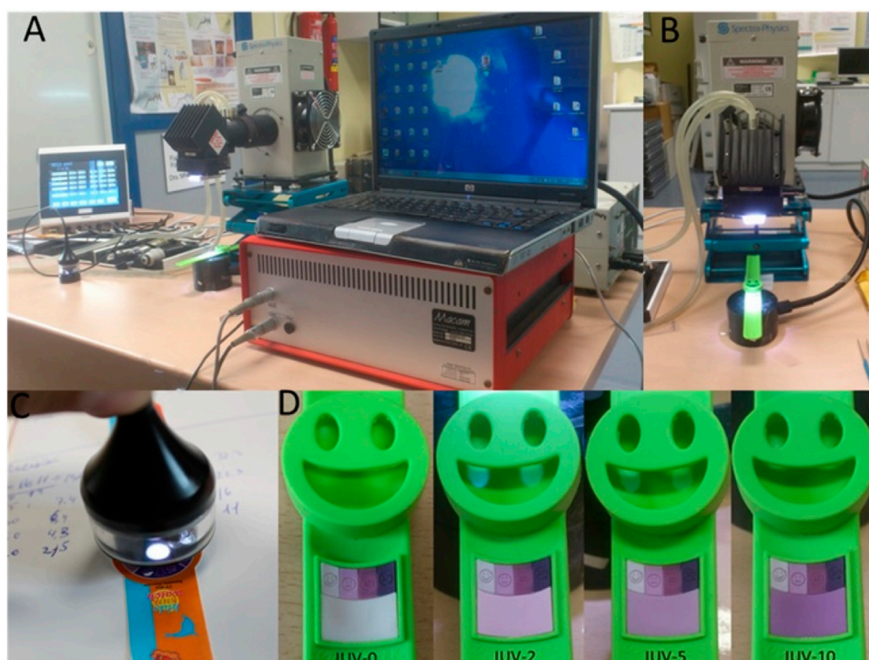
FIGURE 1 (A) Image of the lighting system with solar simulator, spectral measurement system, and colorimeter. (B) Illumination of photochromic wristbands under solar simulator. (C) Color intensity measurement. (D) Purple color of a photochromic wristband under different UVI levels.
