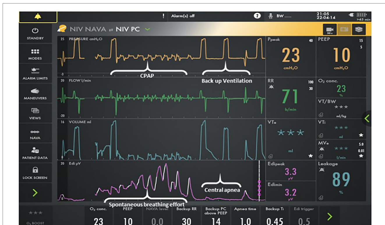
FIGURE 1 Screenshot for the Servo-I ventilator. The bottom line represents the Edi signal. The next lineup is volume, and the third lineup is flow. The top line is pressure. Patient interface resistance compensation in the NAVA software program provides minimal support above CPAP when breathing. Backup ventilation is provided when apneic. Auto-triggering does not occur as neural triggering is the mechanism for initiation.
