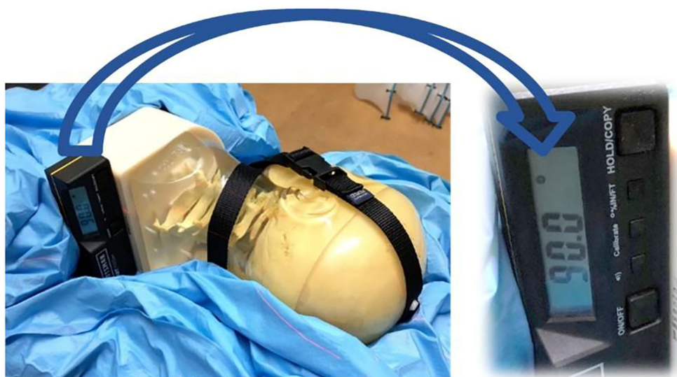
FIGURE 1 Ensure that phantom can be rotated to a specific angle and that it can maintain this position through immobilization measures.
