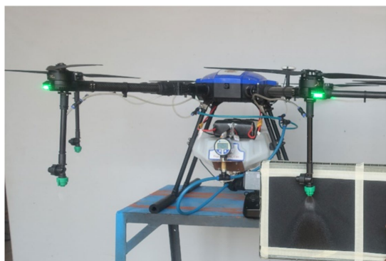
FIGURE 6 Experimental layout for measurement of spray angle.
