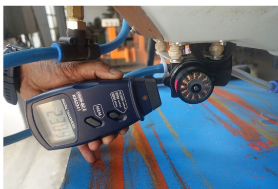
FIGURE 5 Experimental layout for measurement of spray motor speed.
