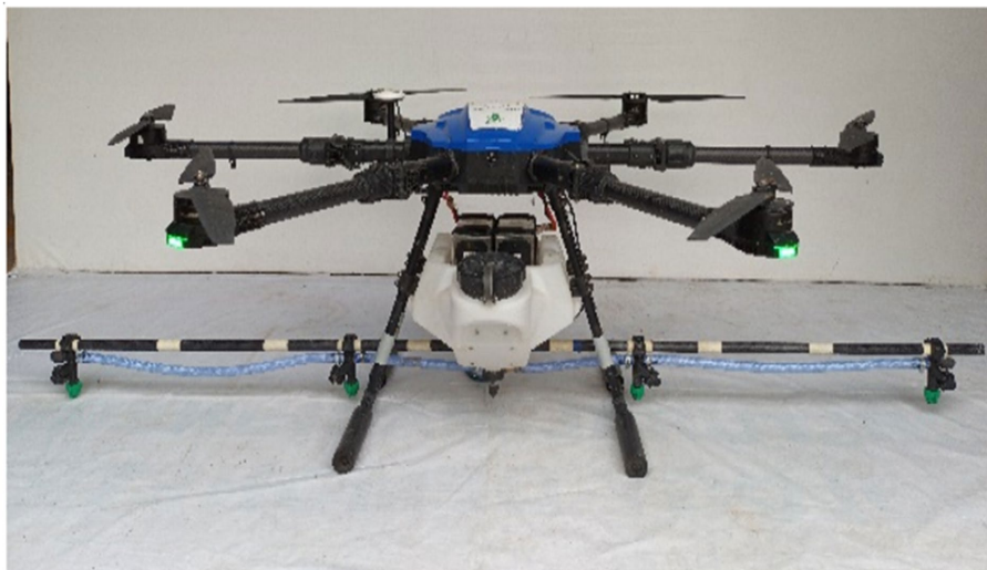
FIGURE 16 Arrangement of spray nozzles on boom configuration and attachment to Drone sprayer.
