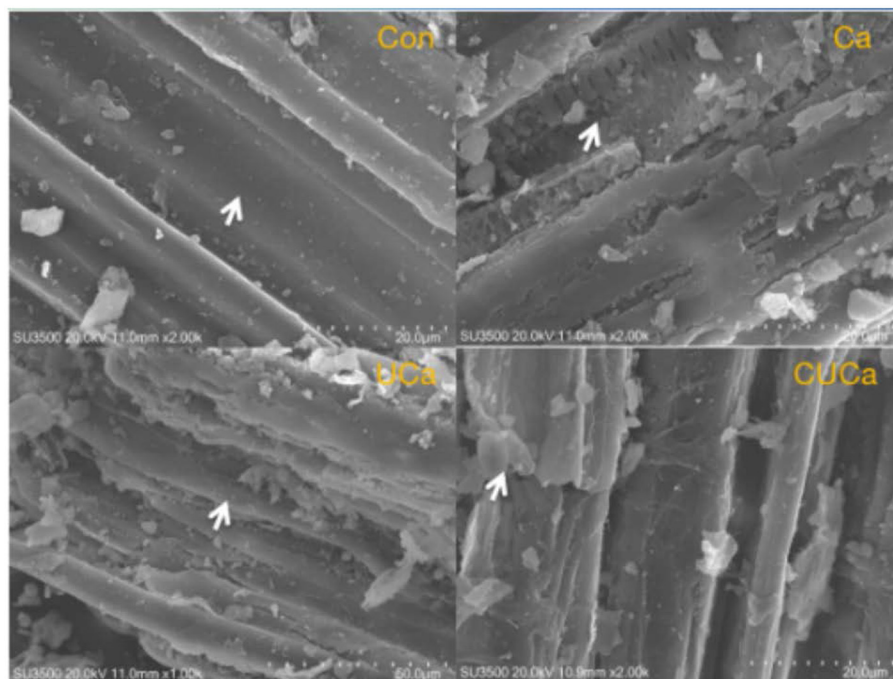
FIGURE 4 SEM images of biomass residues obtained from pretreatment with CSL plus urea-alkali. Con: no pretreatment for control group, Ca: 4% CaO, UCa: 2.5% urea + 4% CaO, CUCa: 9% CSL + 2.5% urea + 4% CaO. Sample (Ca, UCa, CUCa) showing a coarse surface indicated as arrow, and sample Con displaying a flat face.
