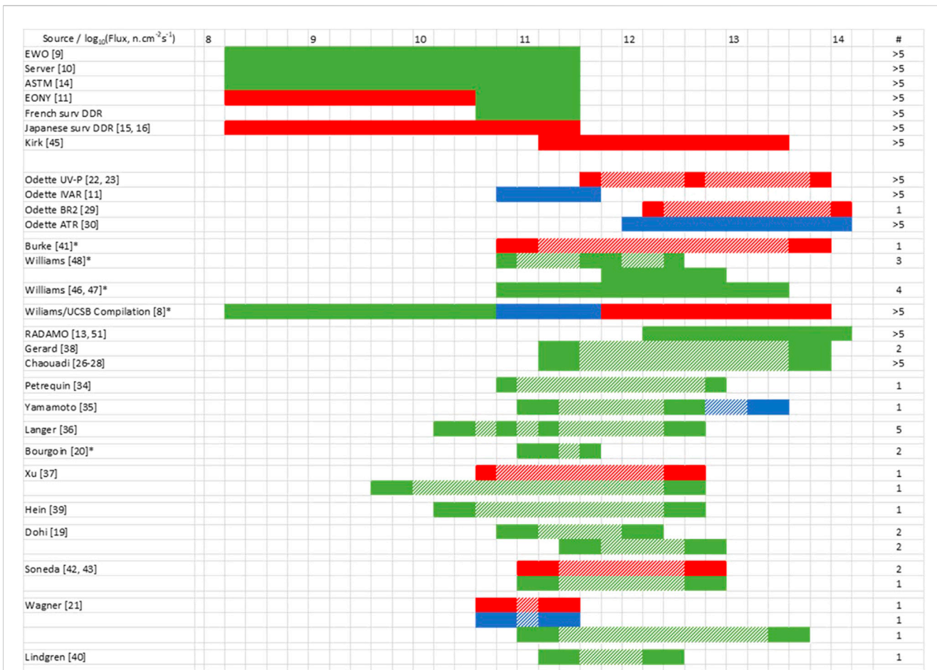
FIGURE 5 Summary of observations on low-Cu steels. Most observations were made at 270°C–310°C. Those marked with an asterisk (*) involved lower irradiation temperatures.
