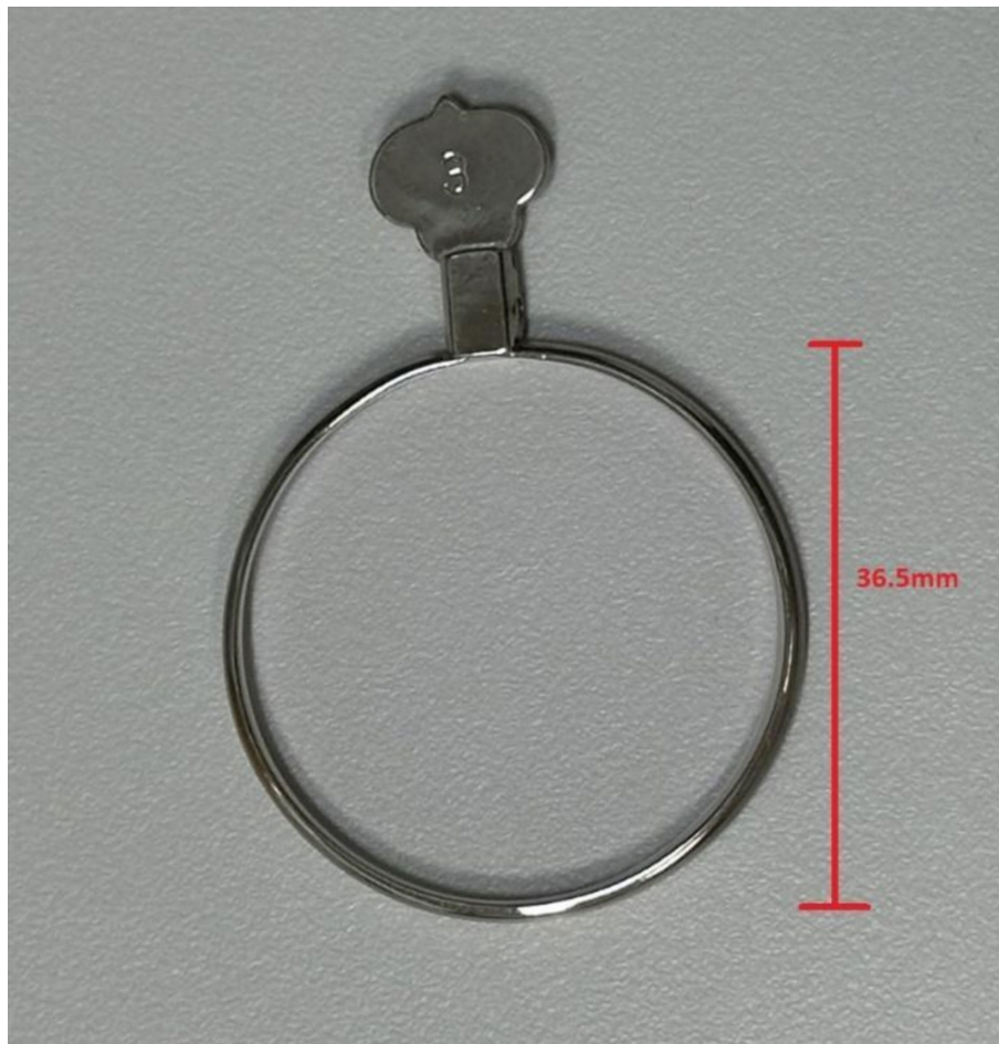
FIGURE 5 The edged DIMS fitted in to a 36.5 mm diameter trial lens ring.
