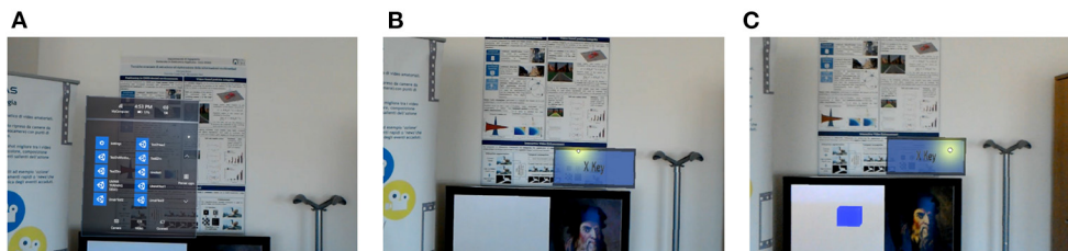
FIGURE 2 Mixed Reality Simple Reaction Time User Interface, showing (A) the device menu prior to starting the test, (B) the X-KEY button, and (C) one of the visual stimuli and the X-KEY button being selected by the user.
