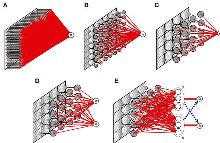
**FIGURE 13** | Description of the different network topologies tested. In **(A)**, the nMNSD is fed with the original image ( $28 \times 28$  pixels); in **(B)**, the pixels are grouped in 49 ( $7 \times 7$ ) fields; in **(C)**, the pixels are grouped in 16 ( $4 \times 4$ ) fields. one-versus-one (OvO); **(D)** Original configuration and **(E)** enhanced version (with inhibitory bundles in blue).
