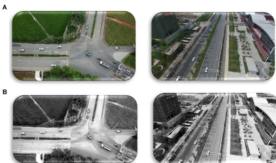
FIGURE 2 Histogram Equalization results over the VAID and Uavid datasets: (A) original Images; (B) Equalized images.
