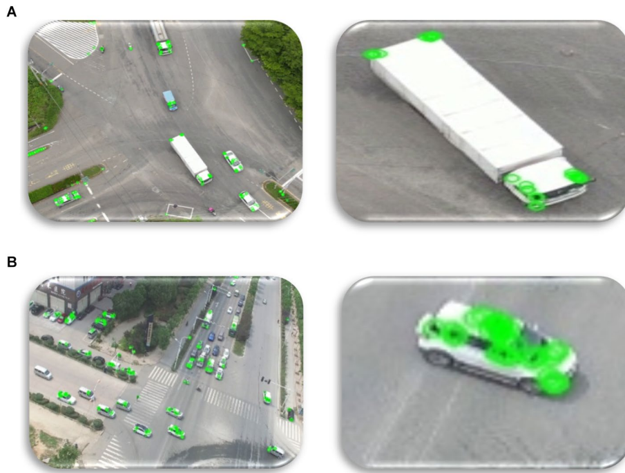
FIGURE 8 Using ORB for feature extraction over (A) VAID dataset and (B) UAVID dataset.
