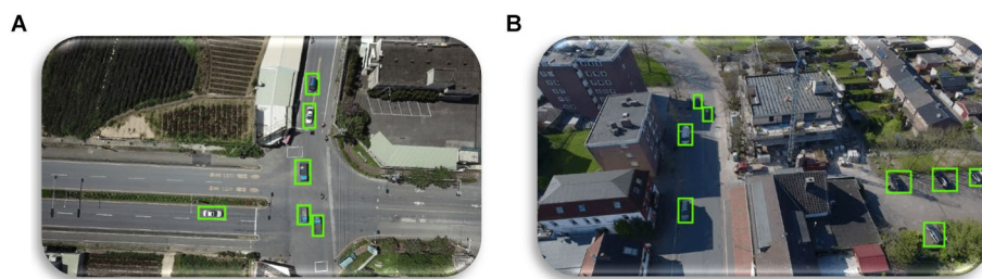
FIGURE 5 Vehicle Detection across (A) VAID and (B) UAVID datasets highlighted with green boxes using the EfficientDet method.
