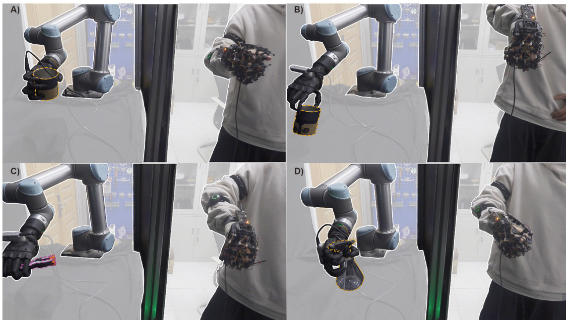
FIGURE 2 Shared control systems can accomplish different kinds of tasks, e.g., interacting with the cup for different functional intent: use (A) and handoff (B); holding the clamp (C); extrusion nozzle of windex bottle (D).
