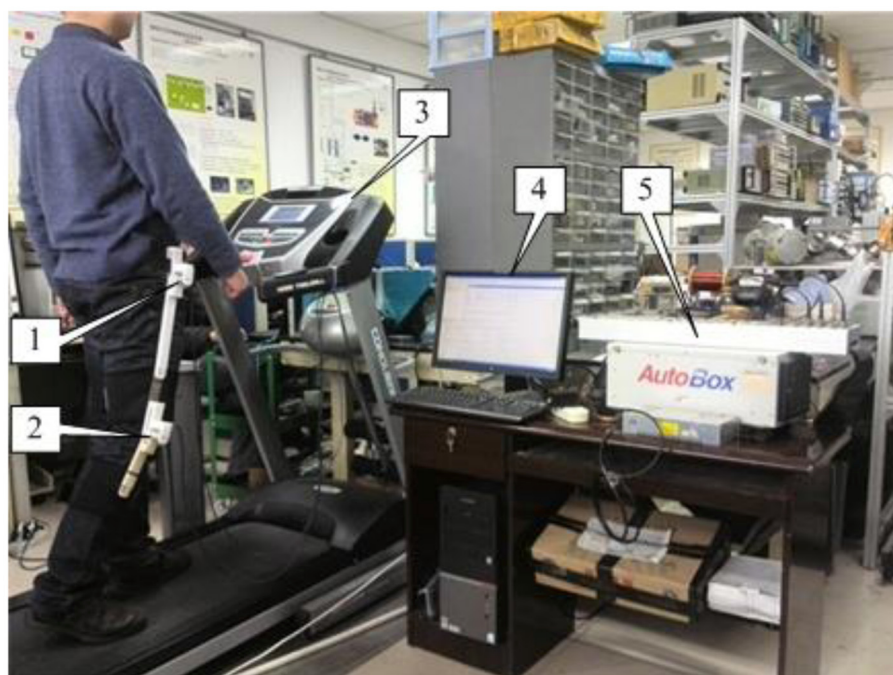
FIGURE 10 Test platform updated from Wang et al. (2013) [1-angle sensor (AS3); 2-angle sensor (AS4); 3-treadmill; 4-PC; 5-dSPACE DS1103].
