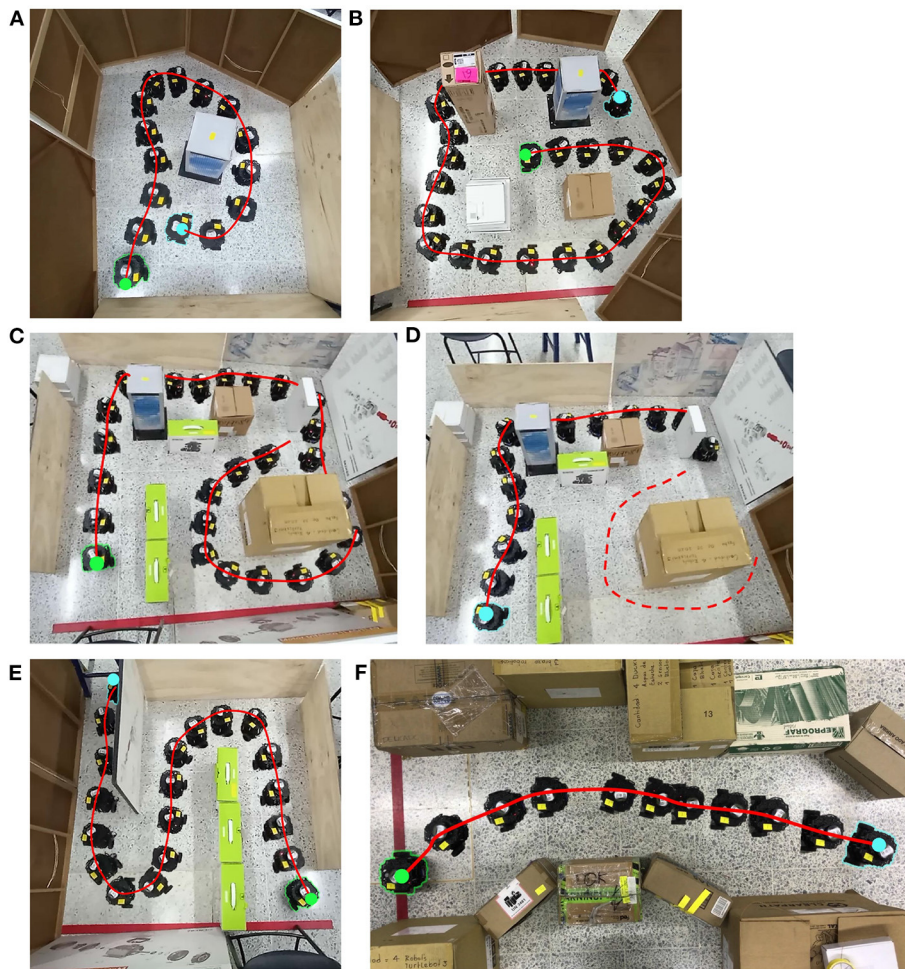
FIGURE 12 Implementation environment results. The path made by the automaton was drawn with red lines in each type of environment. Green circles are initial positions and blue circles are final positions. (A) Loop. (B) Cross. (C, D) Traditional maze part 1 and part 2, respectively. (E) Zigzag. (F) Simple maze. There one can be observed how the automaton completed the (A, E, F) environments successfully. In the (B) environment the automaton’s performance started in the middle of the cross-environment and finished doing circles around the environment. In the (C, D) environments, there can be observed how the automaton’s trajectory finishes at its starting point.
