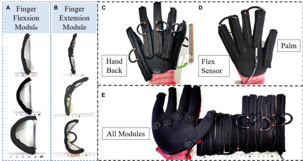
FIGURE 3 Design of a soft hand exoskeleton actuated by SMA-based soft composite structure. (A,B) Finger flexion and extension modules; (C,D) the design of the back and palm of the soft hand exoskeleton; (E) the modular design of the soft hand exoskeleton.
