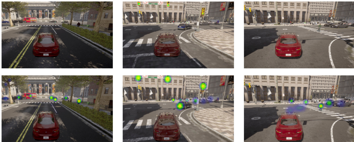
FIGURE 6 Visual attention. The first row is the original image. The second row is the attention image. The dual-flow network focuses on areas near vehicles, pedestrians, and traffic lights.
