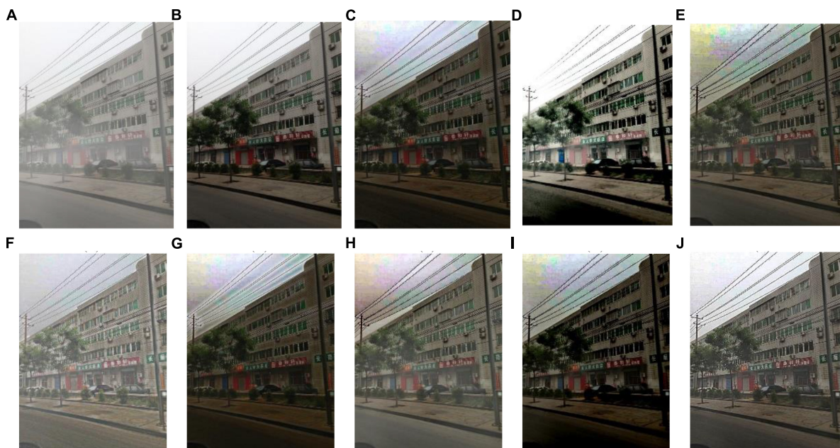
FIGURE 8 Experimental results of different methods for Figure 1 : (A) input image; (B) ground truth; (C) dark channel prior; (D) Fattal et al.; (E) Meng et al.; (F) Tarel et al.; (G) Ehsan et al.; (H) Berman et al.; (I) Raikwar et al.; (J) proposed.
