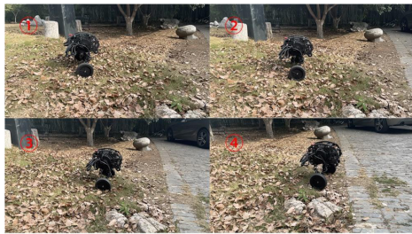
FIGURE 22 Moving over potholed ground.
