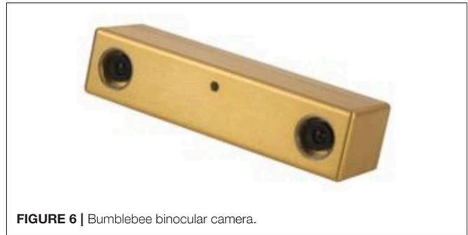
**FIGURE 6** | Bumblebee binocular camera.
