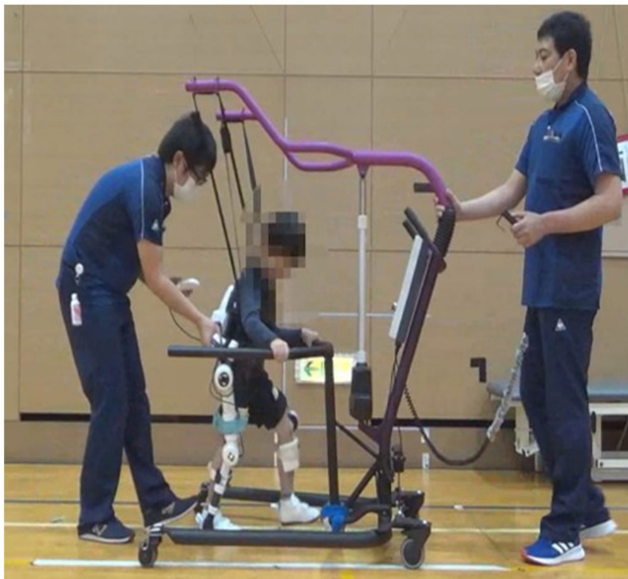
FIGURE 1 Neurorehabilitation using Hybrid Assistive Limb (HAL) of 2S size for a pediatric patient.
