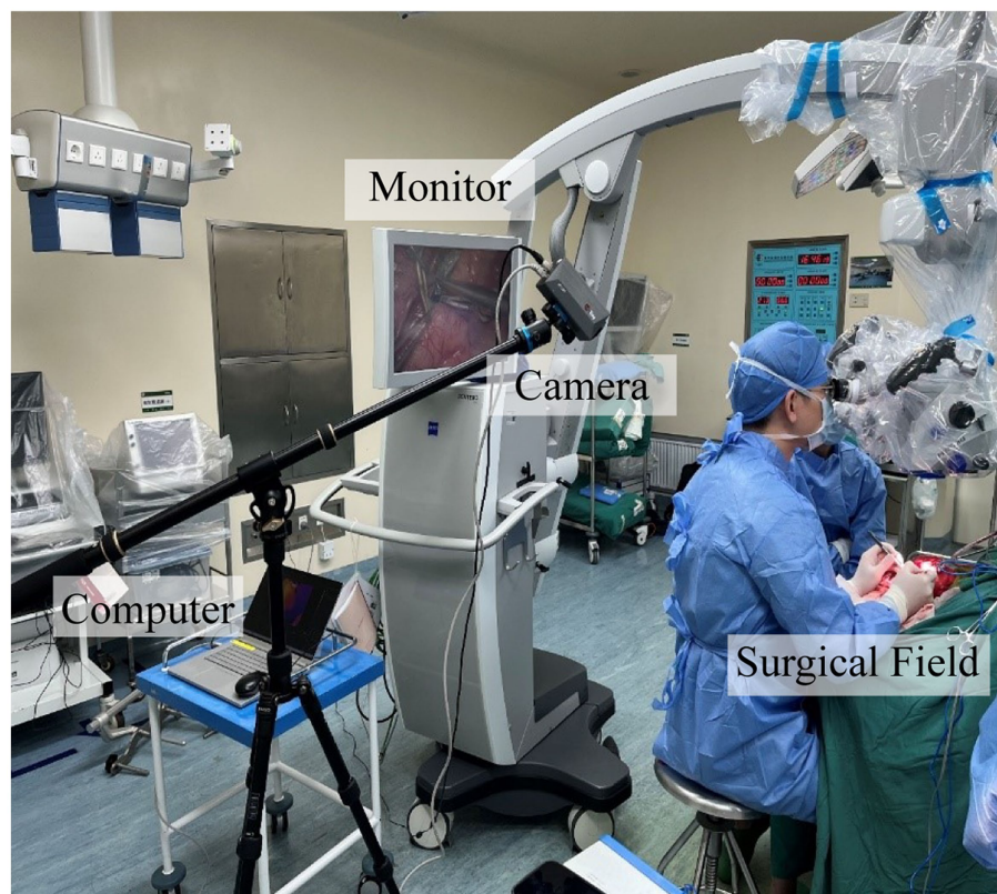
FIGURE 1 Photograph of the infrared imaging system in the operating room.
