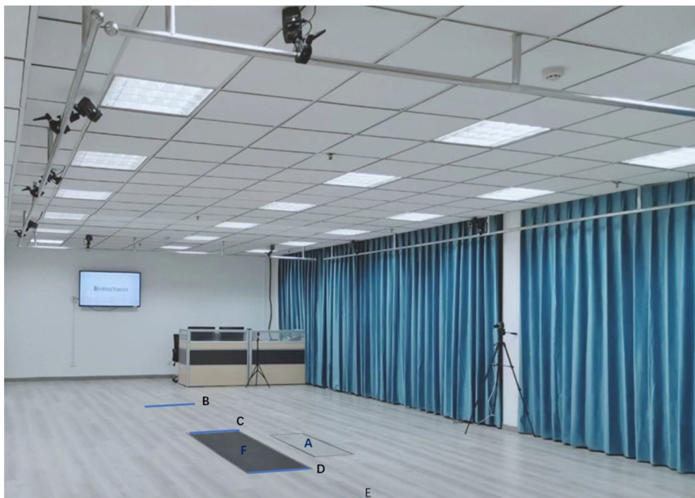
FIGURE 1 Experimental setup. (A) Plantar pressure plate A. The distance between line (B) and (C), line (C) and (D), line (D) and (E) is 2 meters. (F) Plantar pressure plate F.
