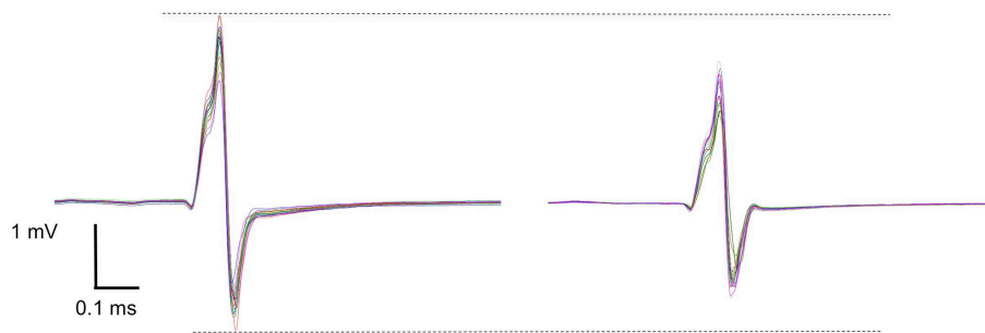
FIGURE 2 | A raw data set of one subject shows the effect of before ( left ) and after ( right ) the rPMS. Each graph shows 15 peak-to-peak superimposed compound muscle action potential (CMAP pp ) curves that were induced by a reflex hammer impact on the Achilles tendon. Mean CMAP pp amplitudes were ~4.2 mV at baseline and ~3.5 mV after the rPMS in this subject.
