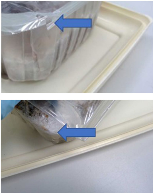
FIGURE 1 Shattered rigid plastic packaging and open film seal from samples from two different brands of RMD.
