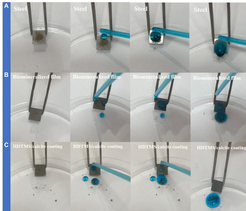
FIGURE 9 | Self-cleaning properties on (A) steel, (B) biomineralized film, and (C) HDTMS/calcite coating by using methylene blue and soil.
