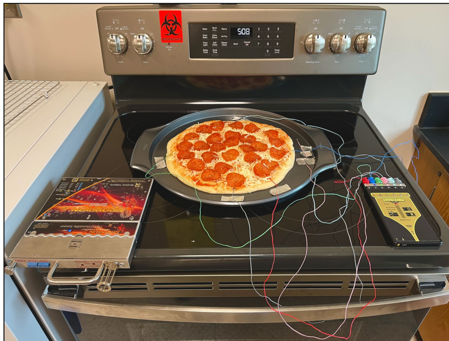
FIGURE 1 Pizza baking validation study setup.
