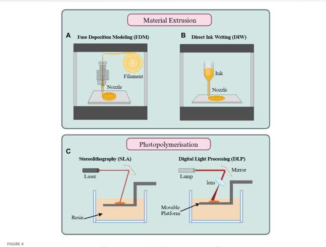
Approaches for 3D printing of membranes: (A) Fuse deposition (FDM); (B) Direct ink writing; and (C) Photopolymerization.
